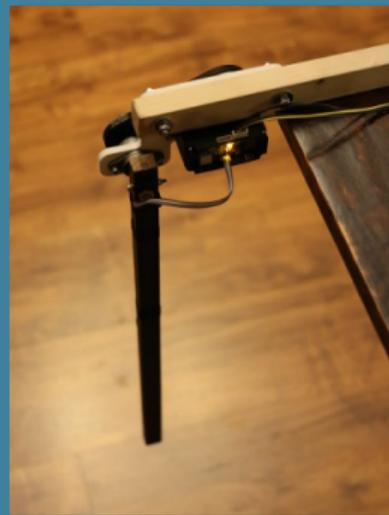
Record motor test data with single leg (pendulum).
